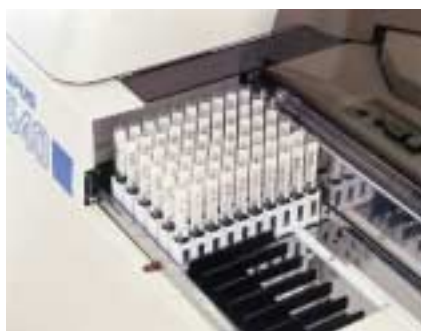
AU 640 sample rack system, already prepared for future automation requests
