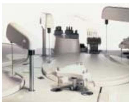
Olympus AU 640 liquid handling components
